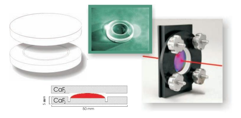
The CaF<sub>2</sub> cell for IR/UV-CD spectroscopy is created between a perfectly flat, optically clear plate and another plate, the center of which is deepened to form a recessed parallel surface surrounded by a groove. This groove serves as a barrier between the sample area and the outer seal, keeping the sample from readily coming into contact with the sealing area. The seal is created by the "upper" flat plate pressing onto the outer ring of the "lower"plate.
