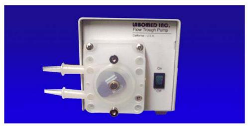
The Flow Through System Pump is fixed-speed, self-priming peristaltic pump. The peristaltic pump roller pressure squeezes fluid through the tubing. The flow is proportional to the speed of the rollers (rpm) and the inside diameter of the tubing).
