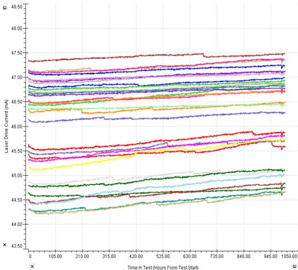
Figure 3 - 60°C 1000 Hour Aging Test
