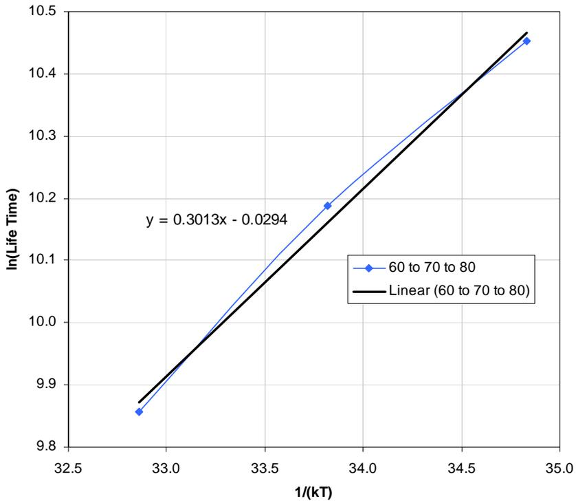
**Figure 6 Three Point Linear Fit of Lifetime Data**
