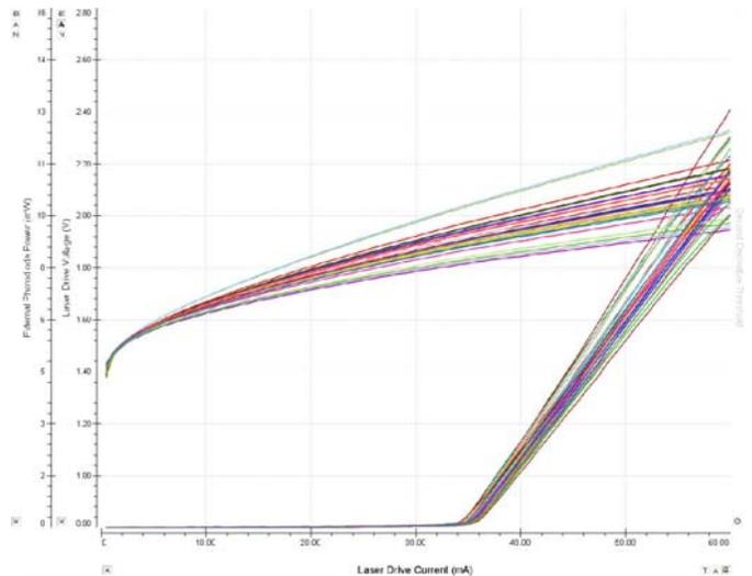
Figure 2 - Post Aging Laser LIV Test Results
