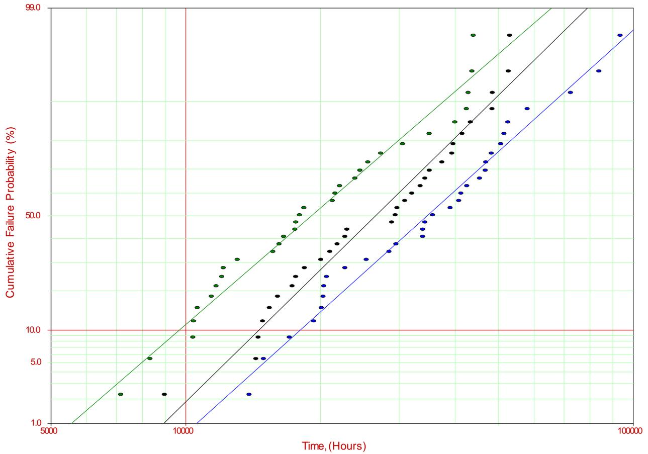
**Figure 5** Lognormal Plots of Times to Failure
