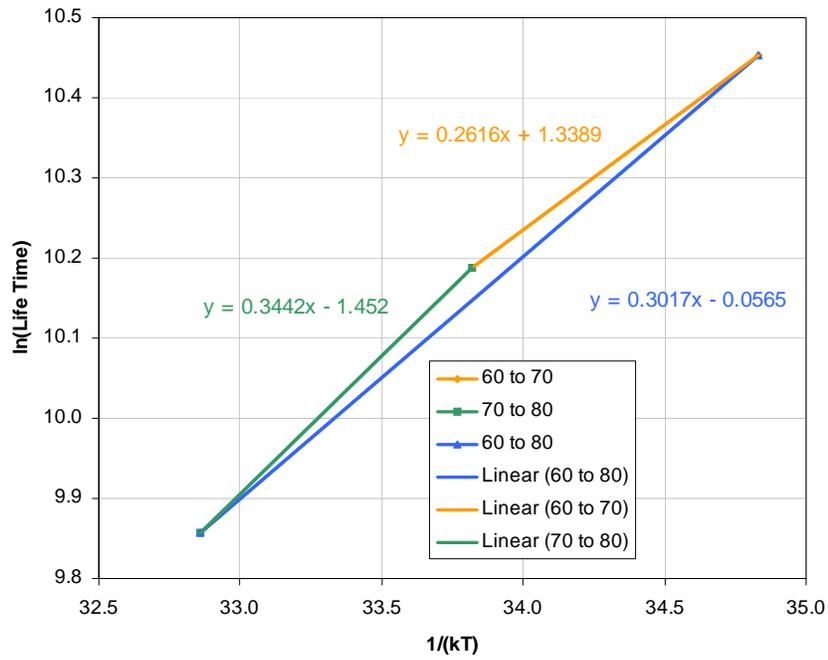
**Figure 7 Two Point Linear Fit of Lifetime Data**
