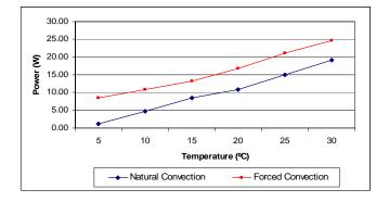
In order to use this data you will need to know a few specifications on your laser diode such as operating current (I), operating voltage (V), and efficiency ( $\eta$ ) of the laser diode. By using the following equation you can calculate the amount of heat that the LDM-4409 will need to dissipate.
