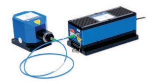
The New Focus VAMP™ series of Tapered Amplifiers is designed to provide up to 2 W of amplified power at a variety of infrared wavelengths. The VAMP will faithfully amplify tunable single-frequency light produced by External Cavity Diode Lasers as well as other light sources of appropriate wavelength.
