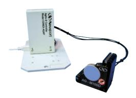
The CONEX-AG-M100D is a piezo motor driven mirror mount with a built-in 2-axis, absolute angle position sensor. The absolute position sensor not only provides highly repeatable positioning, but also enables the recovery of a previously saved position. Utilizing the proven Agilis piezo-motor, direct-drive technology, the CONEX-AG-M100D will hold its position even when the power is turned off. The absolute position sensor enables 0.001° closed-loop MIM and 0.01° bi-directional
