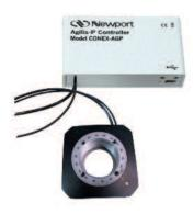
The CONEX-AG-PR100P is a piezo motor rotary stage integrated with a closed-loop piezo motor controller/driver. Initially targeted for repeatable positioning of polarizing optics, it can also be used as a miniature rotation stage for precision positioning of other optics or lightweight samples. The Agilis AG-PR100P rotary stage comes with a built-in direct read encoder, enabling high angular position repeatability. The footprint is maintained while delivering 0.002° uni-directional
