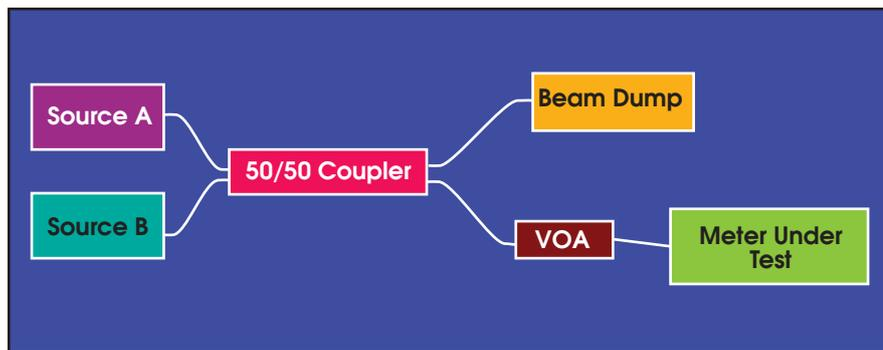
**Figure 2.** A test for linearity typically takes this configuration.
