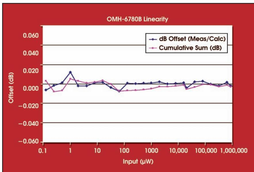
**Figure 3.** Data was taken from 100 nW to 0.1 µW in 3.01-dB steps. This test was run with two 1.0-W SDL 920-nm Fabry-Perot pump lasers. The linearity performance of an ILX Lightwave power/wave head is clearly within the specification of ±0.05 dB.
