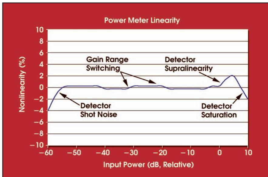
Figure 1. This power meter linearity test shows the combined effects of detector and gain circuit nonlinearities. Power meters in general are designed such that the detector never reaches saturation, which occurs when additional optical input results in a nonlinear response.
