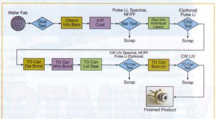
A typical packaging line for a diode laser TO-can features several test steps that offer opportunities for increased efficiency.
