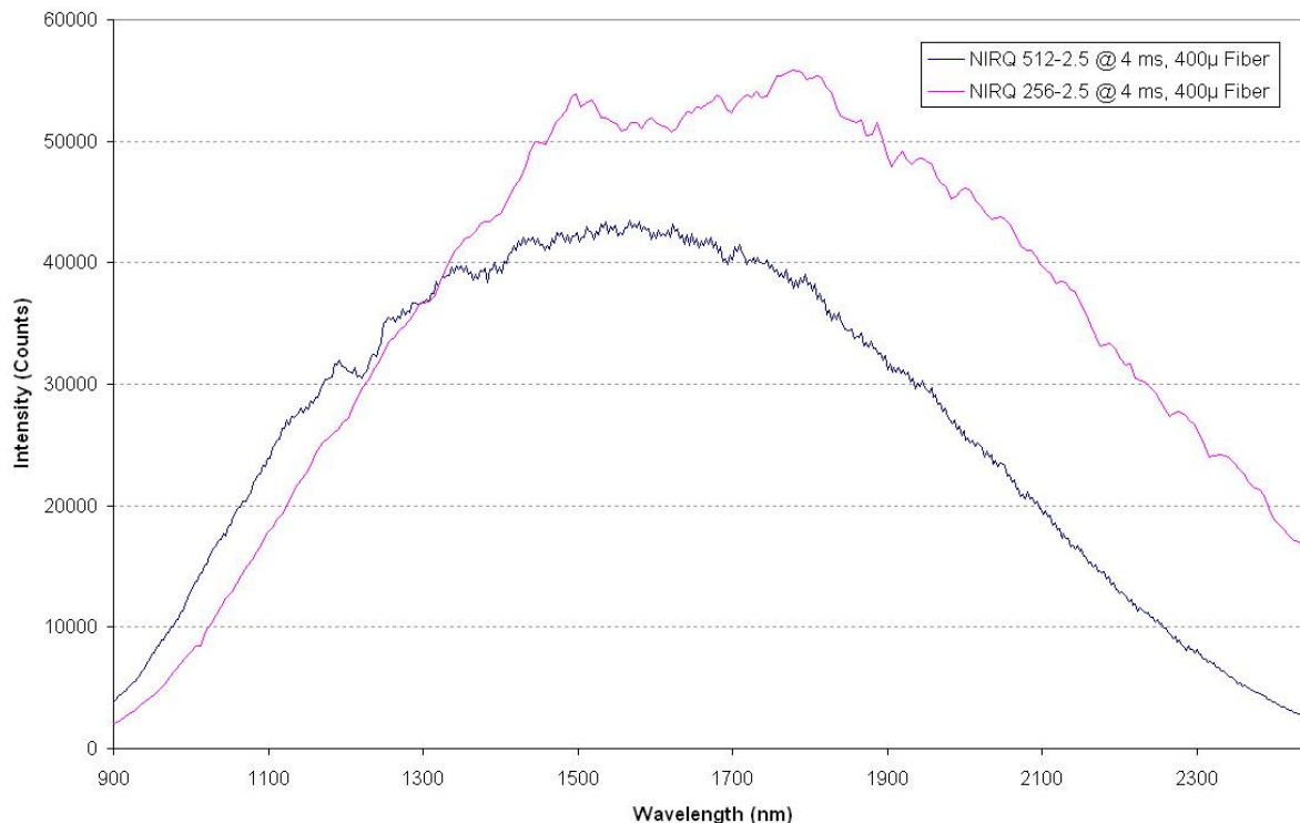
Relative intensity of NIRQuest 512-2.5 and a NIRQuest256-2.5 Spectrometer with a 25µm slit directly coupled to an LS-1 Light Source with a 400µm fiber
