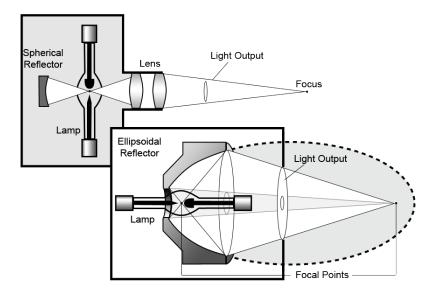
For the same bulb, the OBB PowerArc<sup>™</sup> delivers 5 to 6 times more light, to the secondary focus! That means that an OBB PowerArc<sup>™</sup> lamp housing with a 75 watt xenon lamp provides the equivalent optical power of a 450 watt xenon lamp in an old style vertical lamp housing. And it does so with greater power density due to a smaller focal spot, and at a small fraction of the cost of a big old 450 watt illuminator.
