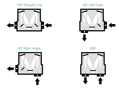
You can also elect as an option to have two entrance ports or two exit ports. This option adds an appropriate flipping mirror(s) and slit assemblies. The flipping mirror is manually switched to receive light from either entrance port, or to deliver light to either exit port depending on the configuration.
