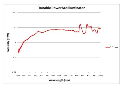
Think of the OBB Tunable PowerArc™ Illuminator as a continuously tunable high intensity laser. It can produce tunable monochromatic light with hundreds of milliwatts of power, and an overall available spectral output from 180 nm to 24 microns.
